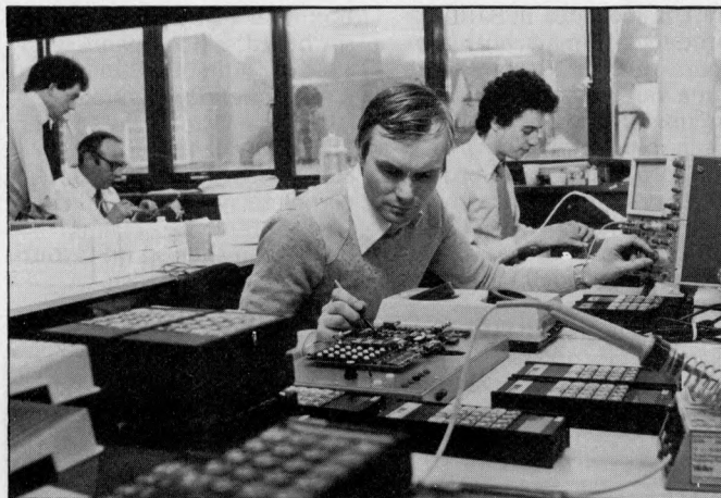
(Bad News. . .) Meter reading terminals under assembly and test at UCSL in Berkhamstead.
